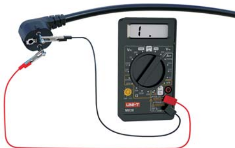
Measurement of the heating core's resistance
