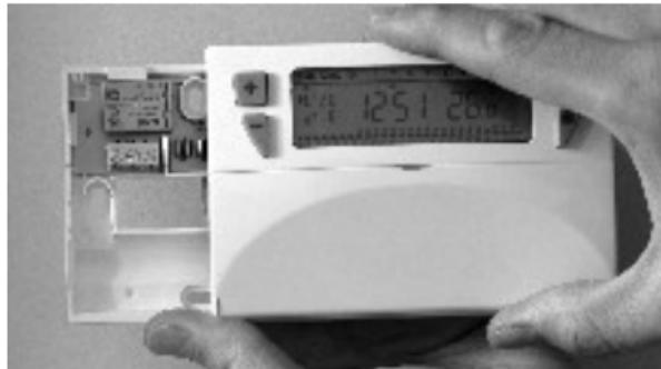
The ELEKTRA DIGI2 (with air sensor) should be installed at least 1.50 m above the ground on an inside wall, protected from direct sunlight, and protected from any heat source (television, lamps etc) and draughts.
